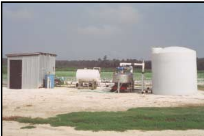
Chemicals can be precision applied to vegetables through a drip system using a stationary chemigation/fertigation system (as shown) or a trailer-mounted system (not pictured).
